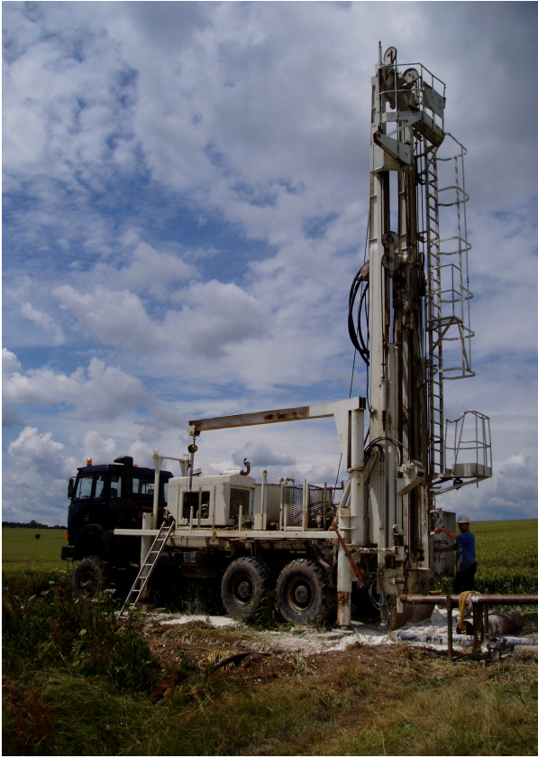
Hydreq Gryphon 16 tonne rotary rig drilling a borehole for a water bottling plant.
